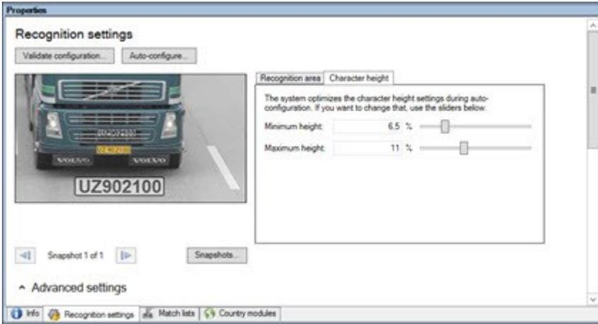
The overlay in the snapshot displays the currently defined character height setting. The overlay grows and shrinks proportionally to the character height settings to the right. For easy comparison, drag the overlay on top of the real license plate in the snapshot. Zoom with your mouse wheel for a closer look.
