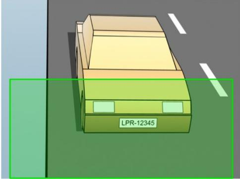
Take a snapshot and make sure that the requirements to stroke width and plate width as described below are fulfilled. Use a standard graphics editor to measure the amount of pixels. When you start the process of reaching the minimum plate width, begin with a low resolution on the camera, and then work your way up in a higher resolution until you have the required plate width.
