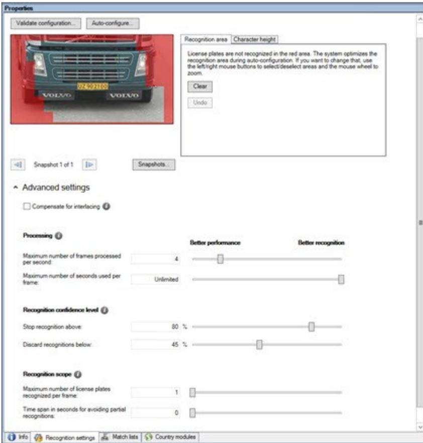
When the optimal results are met, the recognition process stops and returns the license plate it recognized at that point.
