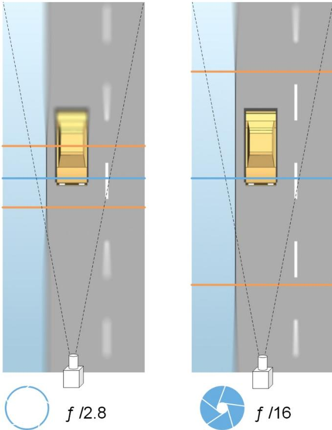
The example illustrates how the depth of field is affected by the f-stop value. The blue line indicates the focus point.
