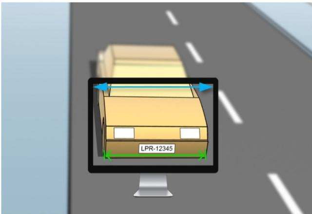
We estimate that the horizontal width is 200 cm/78 inches, as we assume the width of a standard car is 177 cm/70 inches, and besides that we add ~10% for the extra space. You can also do a physical measuring of the area of interest if you need to know the exact width.
