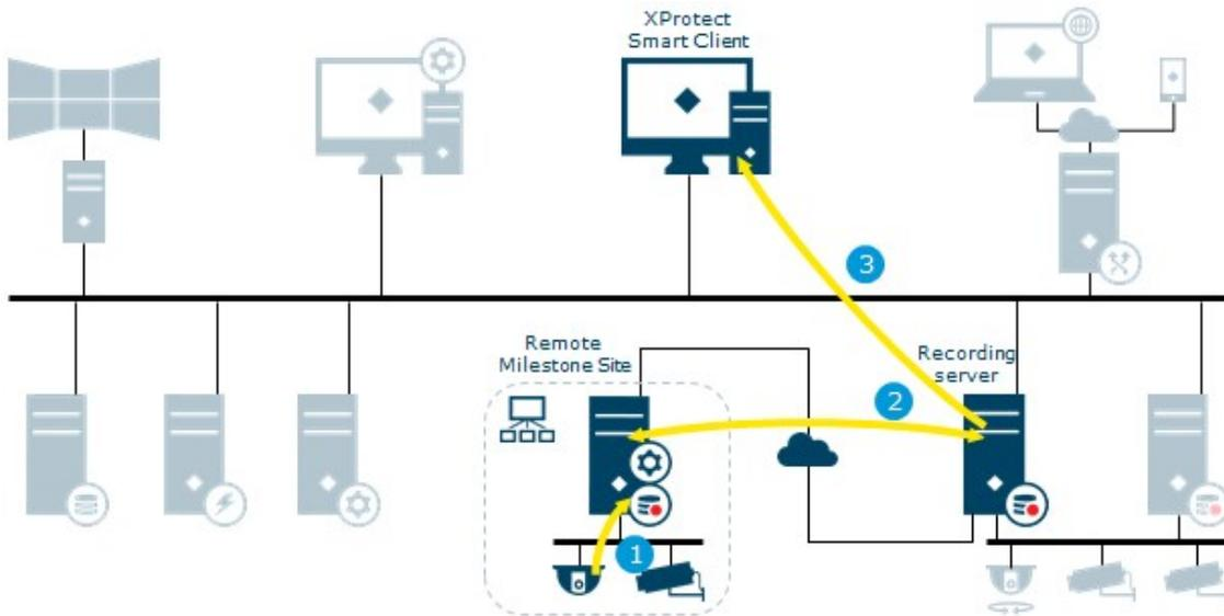
Illustrates how XProtect Smart Client users, specified for the interconnected system, only need to log into the management server on the central site to view video.
