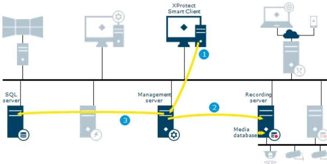
1. The user creates an evidence lock in XProtect Smart Client. XProtect Smart Client sends the information to the management server
