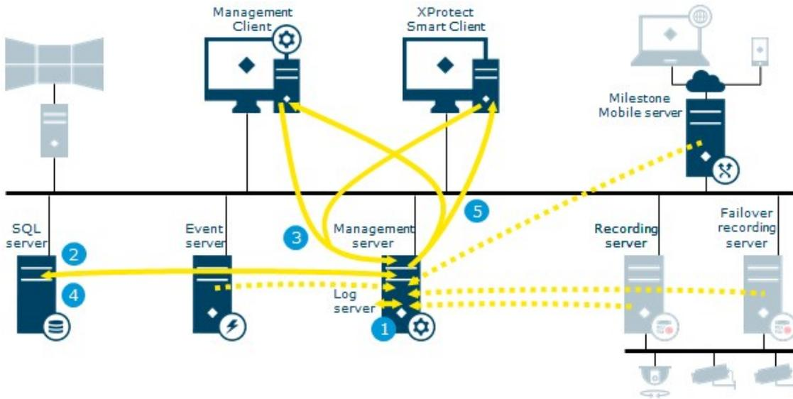
1. System status received on management server delivered by: log server, event server, recording server, failover recording server and mobile server
