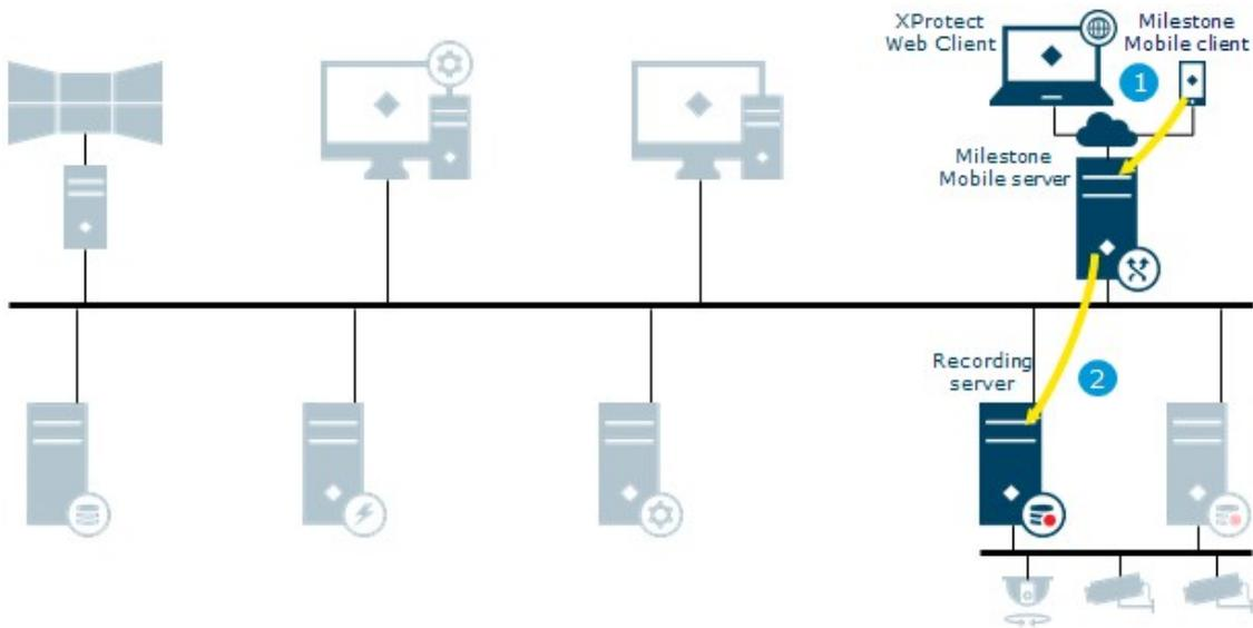
1. Video push stream from a device running XProtect Mobile is sent instantly to the mobile server
