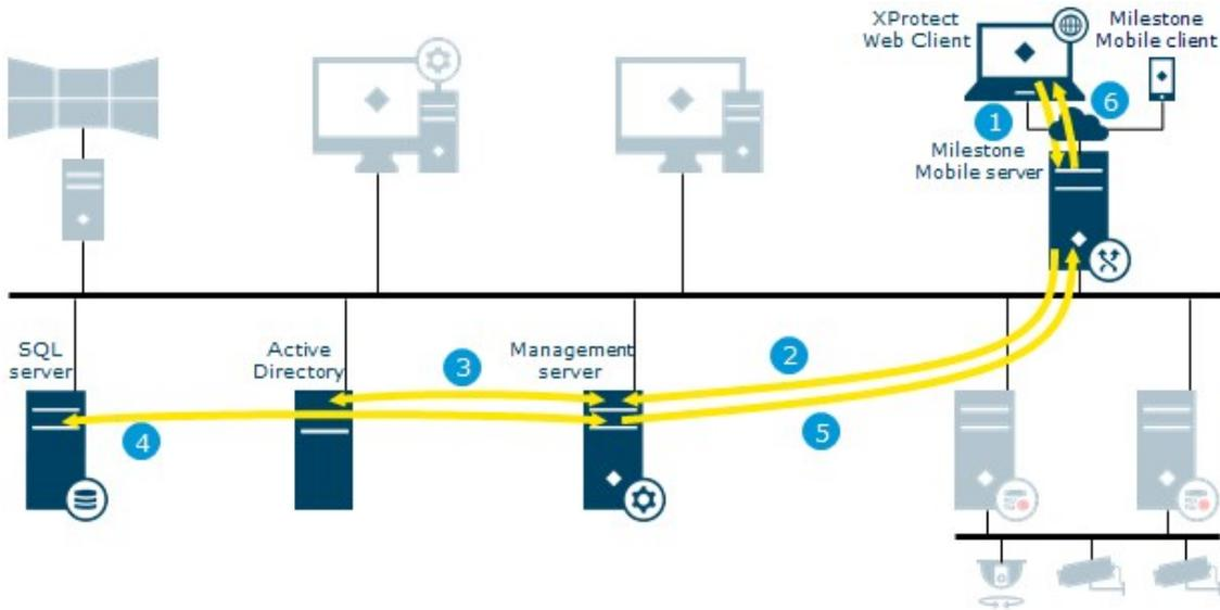
1. Login request from XProtect Web Client or XProtect Mobile received on the mobile server
