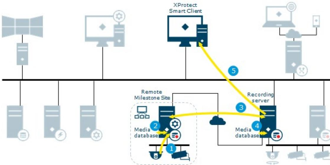
Illustrates when recording is done on both sites. Recordings can be retrieved to the central site based on schedule, event or request. XProtect Smart Client users, specified for the interconnected system, only need to log into the management server on the central site to view video.
